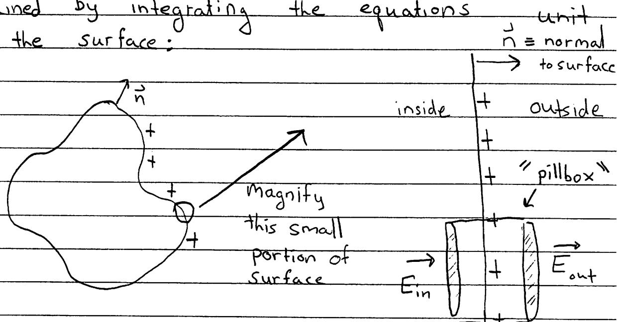
Sufficiently close to the surface it looks like a plane of charge. Applying Gaus Law to the "pillbox" we have
