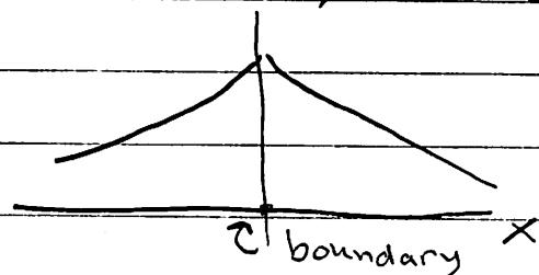
(the E-field) jumps across the surface in proportion to  $\sigma$ .
