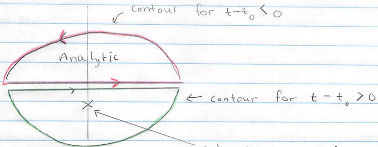
pole at  $\omega = \omega_* = -i\gamma$
