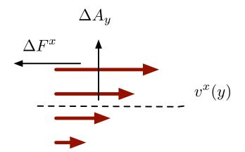
I put a y-index on  $\Delta A_y$  to indicate that area vector we are considering,  $\Delta \vec{A} = \Delta A \vec{n}$ , is pointing in the y direction.
