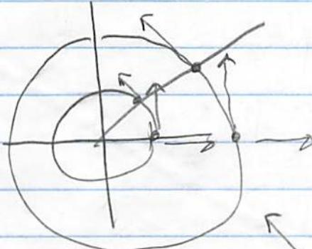
$\partial_\phi \vec{g}_\phi$  is the acceleration of a particle going round a circle. The acceleration points inward.
