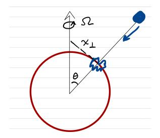
(a) Determine the moment of inertia tensor around the new center of mass of the sphere+meteor after the impact. Take the z axis as the line connecting the center of the sphere and the meteor, and the x-axis parallel to  $x_{\perp}$  line as shown in the figure.
