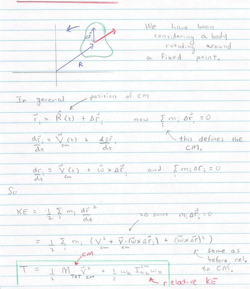
Similarly if the center of mass is moving  $(L) = (R \times (M\vec{v})) + I^{cm} \omega^{b}$ a-th component of angular momentum around O The upshot? In many cases e.g. tumbling of a mechanics book in free fall the wobble of the earth's etc. We can neglect the effect of gravity and the CM motion. It decouples from the free rotations of the body
