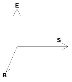
• The magnetic energy per volume stored in the wave is the same as the electric energy per volume stored in the wave
