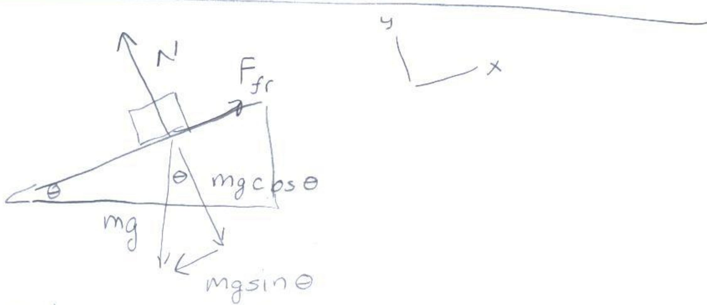
To find the acceleration break up the forces into x and y directions:
