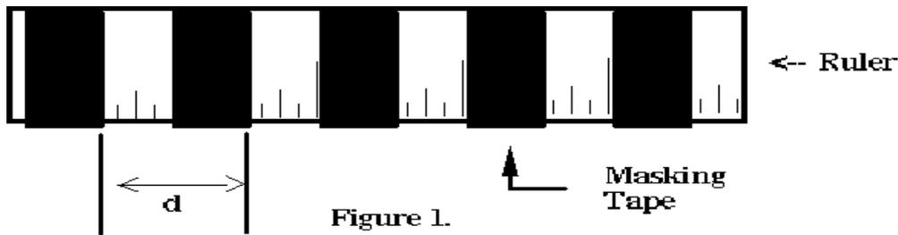
**2. Interval Measurement:** Measure the interval  $d$  between the two successive leading edges of the tape pieces, i.e., one piece of tape and one blank spot (see Figure 1). To do it more accurately measure the distance from the first leading edge to the last one and divide it by the number of intervals between them.
