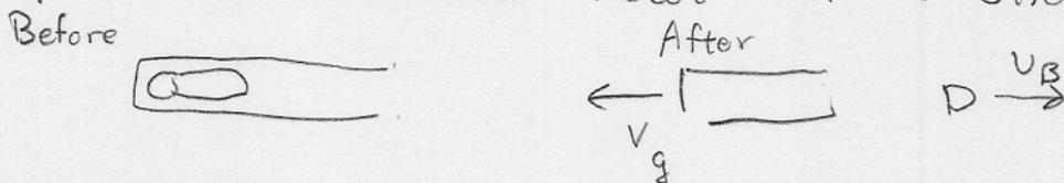
$$P_{\text{before}} = 0 = P_{\text{After}} = m_g v_g + m_B v_B$$
