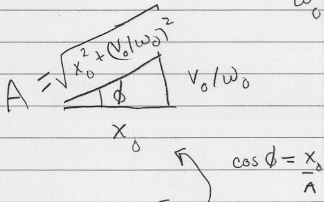
$$A = \sqrt{x_0^2 + \left(\frac{v_0}{\omega_0}\right)^2} \quad \leftarrow \text{will turn out to be the amplic}$$
