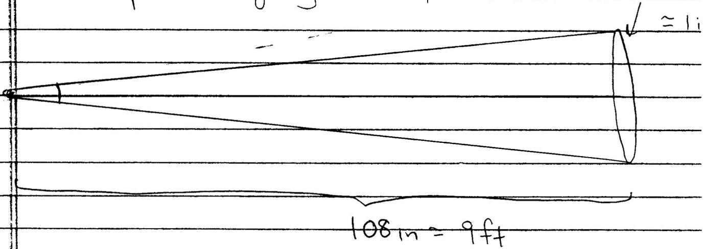
Thus by measuring the conical shape / angle of the shadow can measure the ratio of two distance
