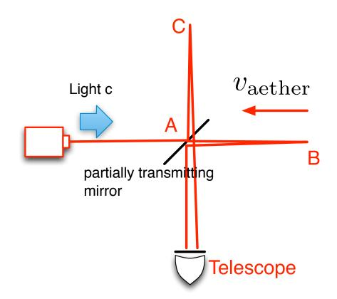
The two beams pass through the (two-way) mirror travel ABA and ACA and recombine in the telescope making an interference pattern
