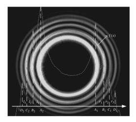
• In general you will always see such an interefrence pattern even without the aether, because the lengths ABA and ACA are not exactly equal. So, how do you tell the effect due to the "aether"? The way you do this is by rotating the apparatus by 45° – In this case the "aether" effect goes away and the interference pattern changes. The change in the intereference pattern would then be unambiguously due to the light's longer time to traverse ABA.
