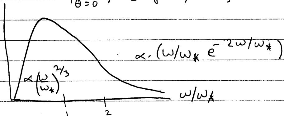
$$2\pi \left. \frac{dW}{d\omega d\Omega} \right|_{\theta=0} = \frac{3e^2\gamma^2}{4\pi^2c} \left( \frac{\omega}{\omega_*} K_{2/3}(\omega/\omega_*) \right)^2$$
