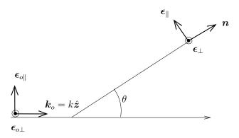
So there are four cases depending on whether the incoming and outgoing polarizations are parallel or perpendicular to the scattering plane. For example, the cross section to produce light of polarization  $\epsilon_{\perp}$  by un-polarized light (50%  $\epsilon_{o\perp}$  and 50%  $\epsilon_{o\parallel}$ ) is
