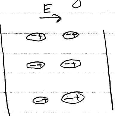
The electric field polarizes the material leading to a net dipole moment/volume proportional to the applied field
