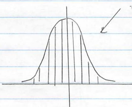
Instead of the original smooth curve one finds a set of spikes separated by  $\frac{2\pi}{T_0} = \Delta\omega$
