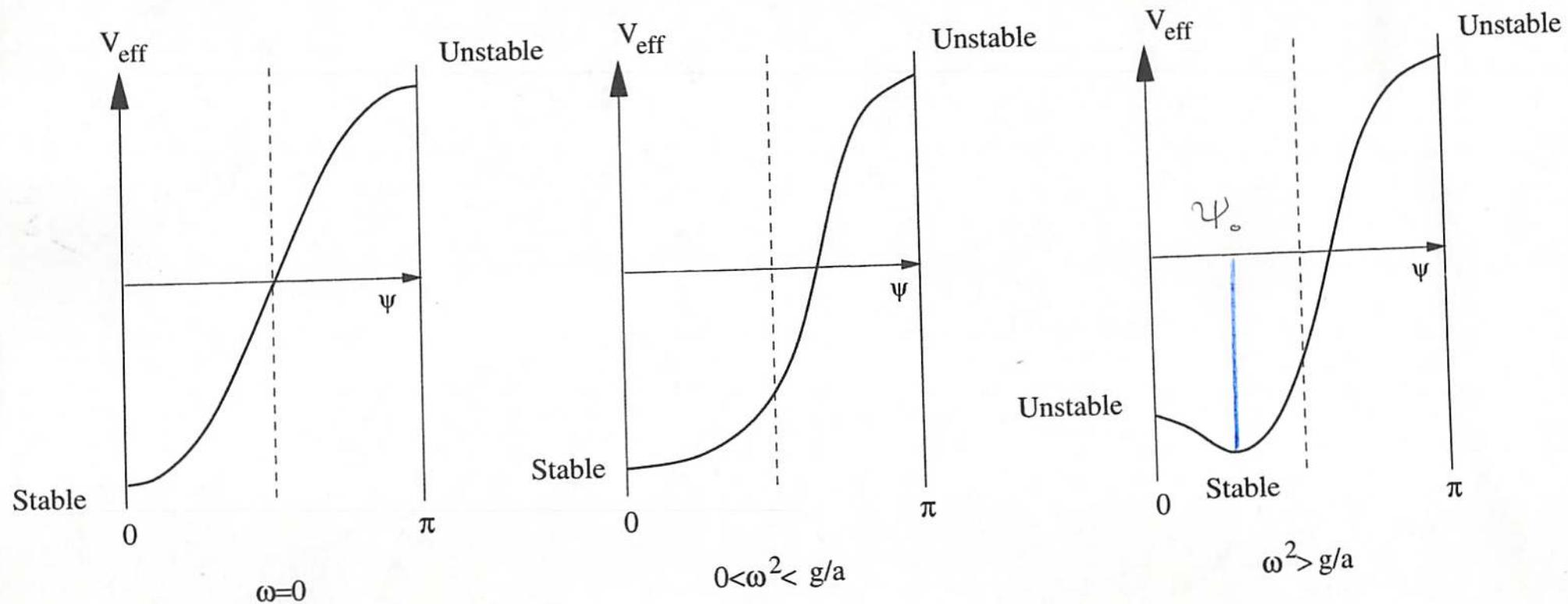
For  $\omega^2 > g/a$  the minimum at  $\psi = 0$  becomes a maximum. The bead will find a new minimum at a finite angle  $\psi_0$ . Physically it is the centripetal force which pushes the bead outward.
