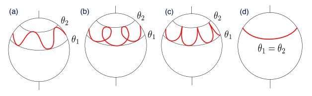
Figure 1: Motion of the tip of the heavy symmetric top
