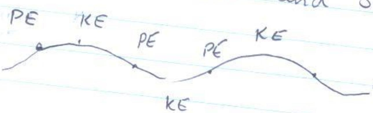
$$\frac{\partial^2 y}{\partial x^2} = \frac{\mu}{T} \frac{\partial^2 y}{\partial t^2} \quad v^2 = \frac{T}{\mu}$$
