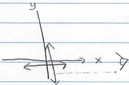
Only the  $y$ -oriented dipole is transverse to the line of sight (the  $x$ -axis)
