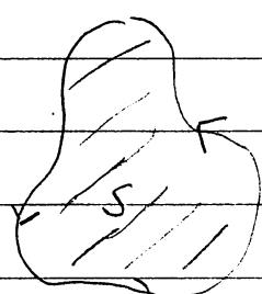
$$\int_S d\vec{S} \cdot (\vec{\nabla} \times \vec{V}) = \int_{\text{loop}} \vec{V} \cdot d\vec{l}$$
